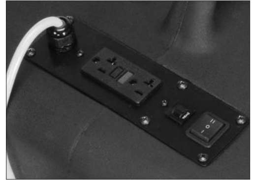
2 position switch and daisy-chained outlets
